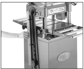
Figure 31. Checking pulley alignment.
